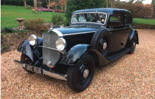
The Mercedes-Benz 200 (W21) was in production from 1933 to 1936, featuring a 2.0-litre straight-six engine, all round independent suspension, and hydraulic brakes. Available in long (3,050mm) and short (2,700mm) wheelbases, this was a 'mid-size luxury car' by the standards of its day.
