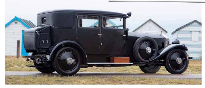
Once the frame, engine, transmission, and axles had been restored and the car brought to rolling chassis state, a replica of the original Gurney Nutting Weymann-type saloon body was fabricated using period photographs as guide. A photograph of '14RF' carrying its original Gurney Nutting body may be found on page 63 of Rolls-Royce The Derby Phantoms by Lawrence Dalton.
