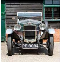
As first conceived, the Frazer Nash chassis employed quarter-elliptic springing, rack-and pinion steering and cable-operated brakes on the rear axle only, though four-wheel braking was soon standardised. The Power Plus 1.5-litre overhead-valve four-cylinder engine was used for the first dozen-or-so cars before the similar-size sidevalve Anzani 4000 series was standardised in 1925.
