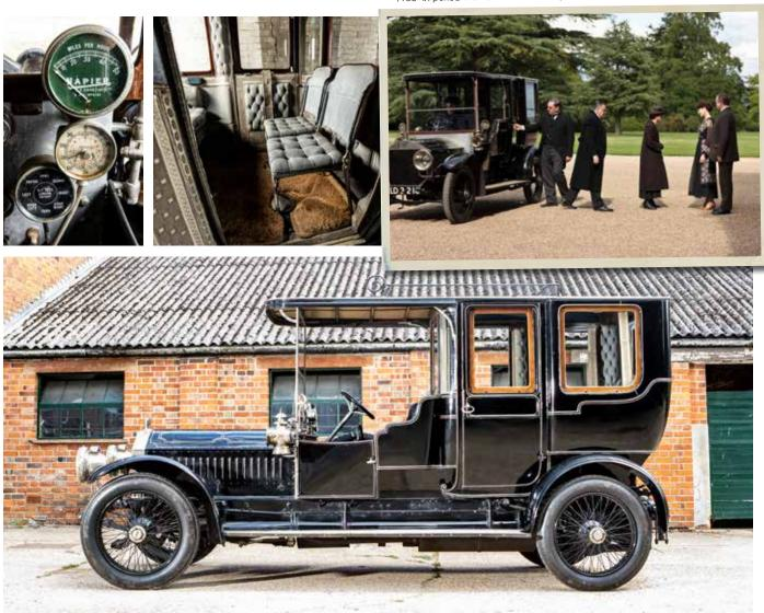
All mechanical work on the chassis and running gear was entrusted to Arthur Archer of Great Dunmow, Essex, who also reproduced the fuel tank and exhaust system. Wheels were rebuilt, brake shoes and drums replaced, patterns made to cast a new water pump, and the electric telegraph from the passenger compartment to the driver repaired. The silk roller blinds have been replaced.
